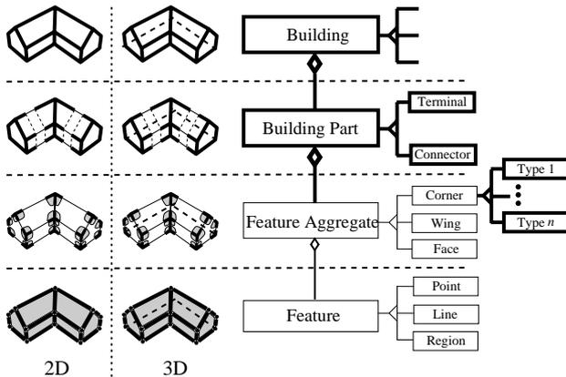
Figure 3: *Component-based building model: The concept 'building' is explicitly represented by the two highest levels and by building specific subclasses and attributes on lower levels. This model extends the general polyhedral model by the bold drawn entities.*
